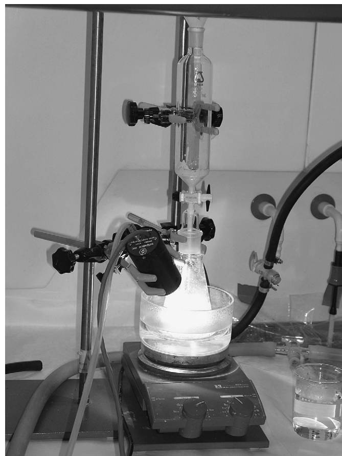
Fig. 2. Device used for fast drying of the starting suspension with the help of a halogen lamp.
