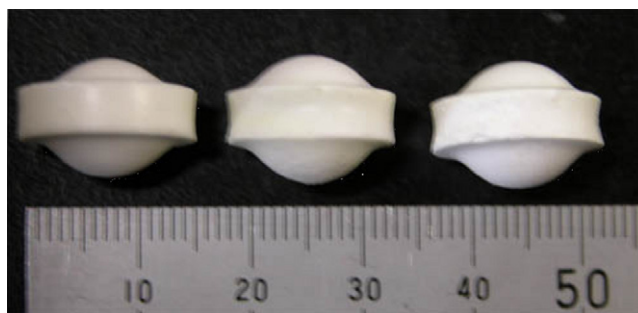
Fig. 1. Side view of macroscopic ceramic foams fabricated by foaming after sintering of zirconia based matrix with silicon carbide as a foam agent (1600 °C holding for 8 h). Foam height: 5.5 mm (left: 3YSZ), 6.5 mm (middle: silica added), 6.2 mm (right: alumina added).
