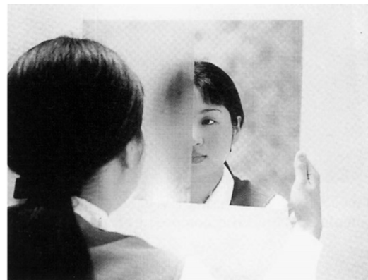
Fig. 2. Anti-condensation effect of a photocatalytic coating.
