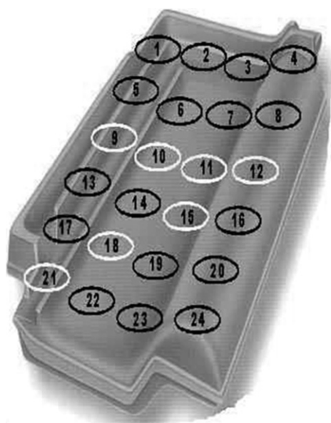
Fig. 1. Schematic presentation of the roofing tile design with the selected tile segments.
