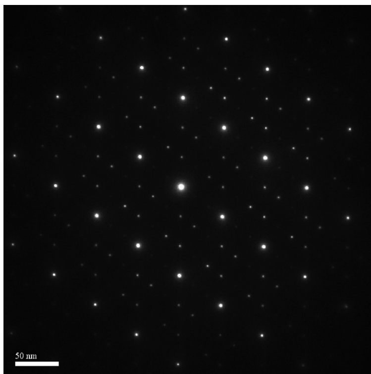
Fig. 5. (1\ 1\ 0)_p zone axis SAD pattern obtained from grains in the sintered specimen with x = -0.01 (diffraction spots at the \{h \pm 1/3, k \pm 1/3, l \pm 1/3\} position arises from the 1:2 LRO on B-site).
