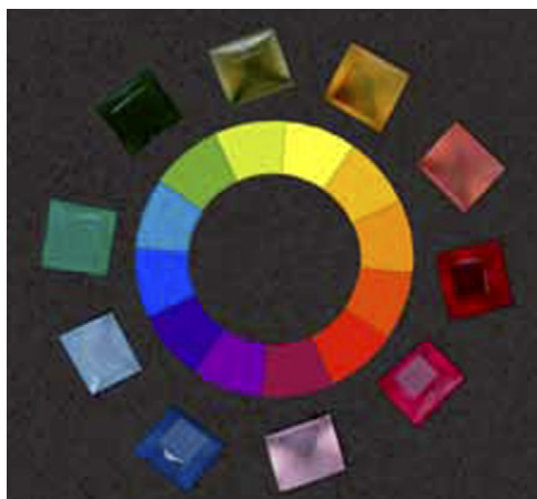
Fig. 15. Transparent sintered corundum ( \alpha - \text{Al}_2\text{O}_3 ) with colours that cover the visible spectrum.
