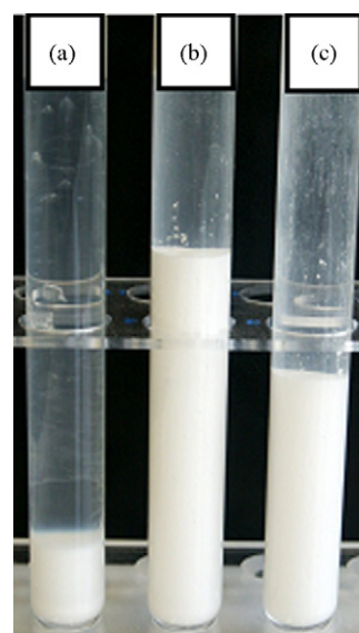
Fig. 2. Picture of 3 vol.% alumina suspensions with (a) no silica and with silica ( \text{mSiO}_2/\text{mAl}_2\text{O}_3 = 1.1\% ) according to the deagglomeration method (b) method 1, (c) method 2.
