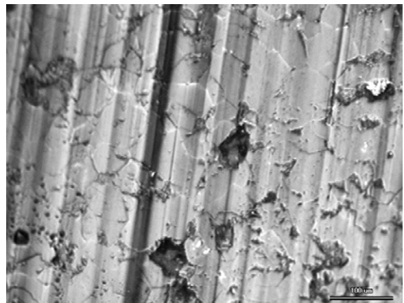
Fig. 14. Optical micrograph showing the worn surface of an alumina ball after sliding against a \text{Si}_3\text{N}_4 -YA coating.
