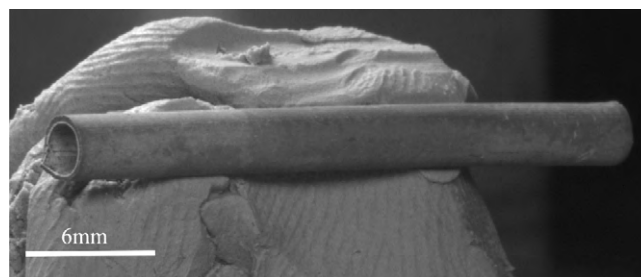
Fig. 19. Longitudinal view of ceramic micro-tube manufactured by co-extrusion showing the inner white YSZ layer surrounded by the four Ni/YSZ layers.
