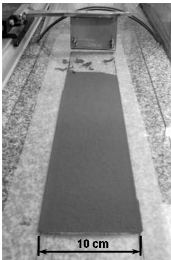
Fig. 6. As-cast tape of doped lanthanum chromite suspensions in ethanol with 55 wt% solids and 15 wt% BS.
