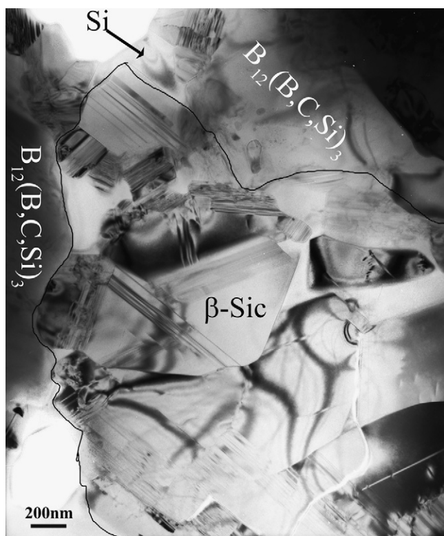
Fig. 5. TEM micrograph of polygonal \beta -SiC particles. These particles consist of several plate-like particles mutually bonded. The contour line marks the polygonal \beta -SiC particle.
