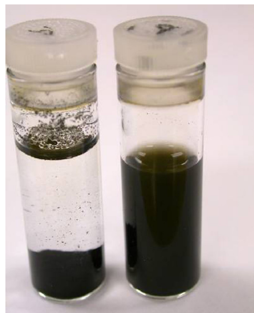
Fig. 2. Settling tests of as-received MWCNTs (left) and purified MWCNTs (right) in water at pH 12.
