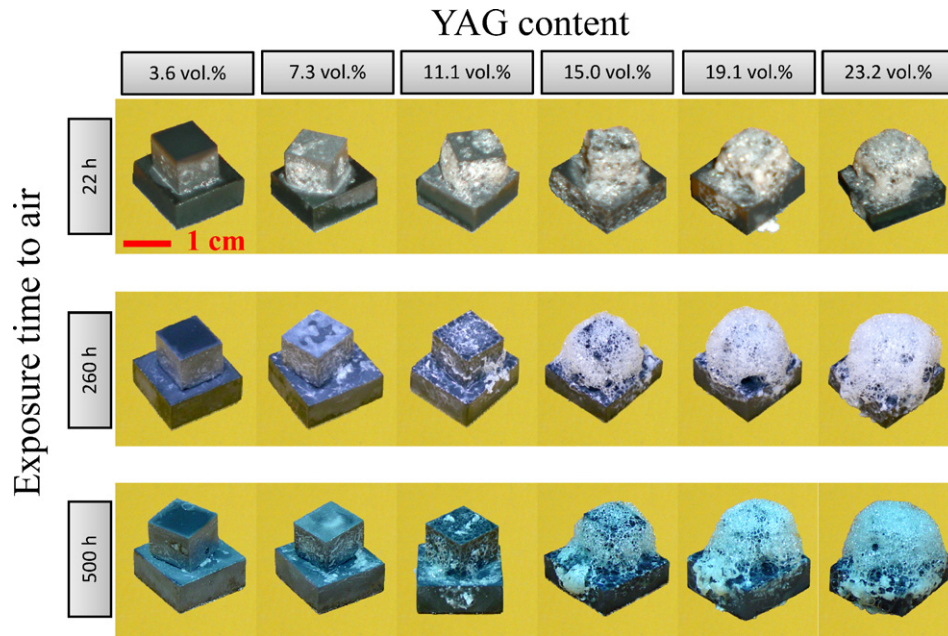
Fig. 3. Surface appearance as a function of vol.% YAG for the PLPS SiC ceramics after oxidation in air at 1500 °C for 22, 260, and 500 h.
