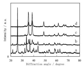
Fig. 4. XRD patterns of microwave irradiated specimen for (a) 0 min, (b) 10 min, (c) 30 min and (d) 60 min at 95  $^{\circ}$ C.
