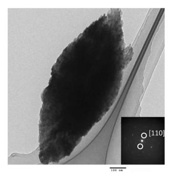
Fig. 6. TEM image and SAED patterns of the leaf-shaped CuO microcrystals synthesized by mantle heater heat treatment.
