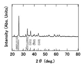
Fig. 1. XRD pattern of the copper precursor synthesized by a homogeneous precipitation.
