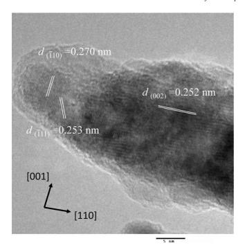
Fig. 7.  $[-1\,1\,0]$  projection of HRTEM image for CuO microcrystal synthesized by microwave irradiation.
