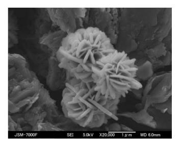
Fig. 2. SEM images of copper precursor particles synthesized by a homogeneous precipitation.
