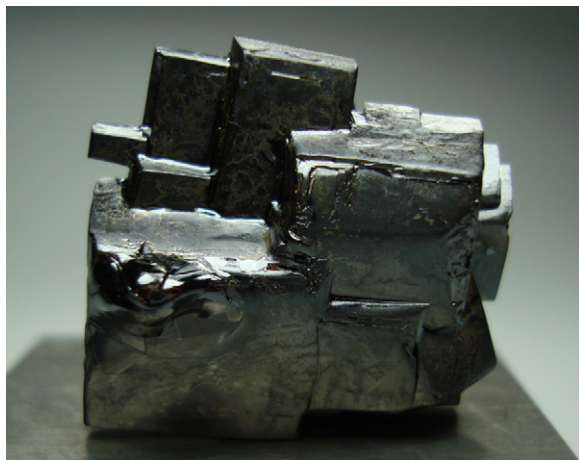
Fig. 3. Single crystals of \text{Bi}_2(\text{Ga}_{1-x}\text{Fe}_x)_4\text{O}_9 obtained using the TSSG single-crystal growth method, with dimensions of 20 \times 20 \times 10 \text{ mm}^3 .
