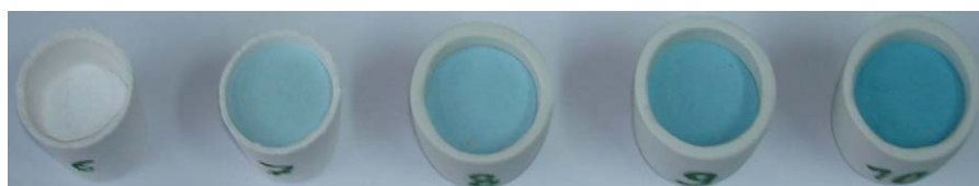
Fig. 4. Images of samples 6–10 after annealing at 1000 °C for 3 h.
