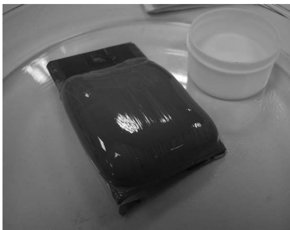
Fig. 2. As-deposited SiC green part.
