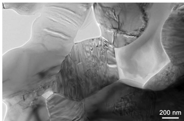
Fig. 7. Transmission electron micrograph of a crystallized EP1.
