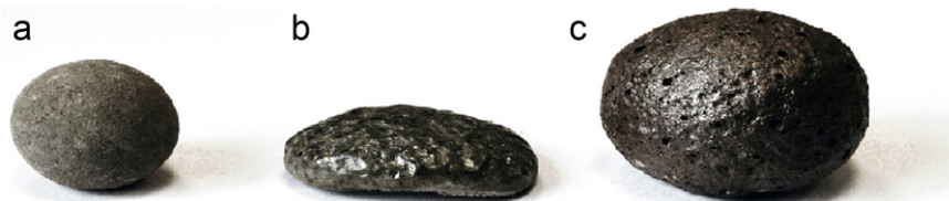
Fig. 6. View of the aggregates: (a) green aggregate. Aggregates sintered at the temperature of 1170^\circ\text{C} , (b) the comparative aggregate made from clay with no added NMP and (c) the aggregate made from clay with NMP (9%).
