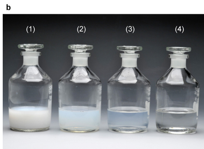
Fig. 4. (a) Particle size distribution of the different coating liquids used in this work. (b) Coating liquids: (1) 85 nm nano-dispersion; (2) 60 nm nano-dispersion; (3) 35 nm colloidal sol; (4) 6 nm polymeric sol.
