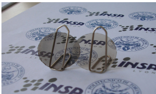
Fig. 10. Sample from US powder, sintered at 1350 °C, before (left) and after (right) annealing at 800 °C for 1 h in air. The two samples are 1.4 and 1.3 mm thick.
