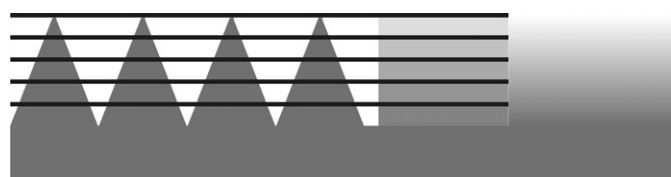
Fig. 5. Schematic representation of refractive index from pyramidal surface pattern.
