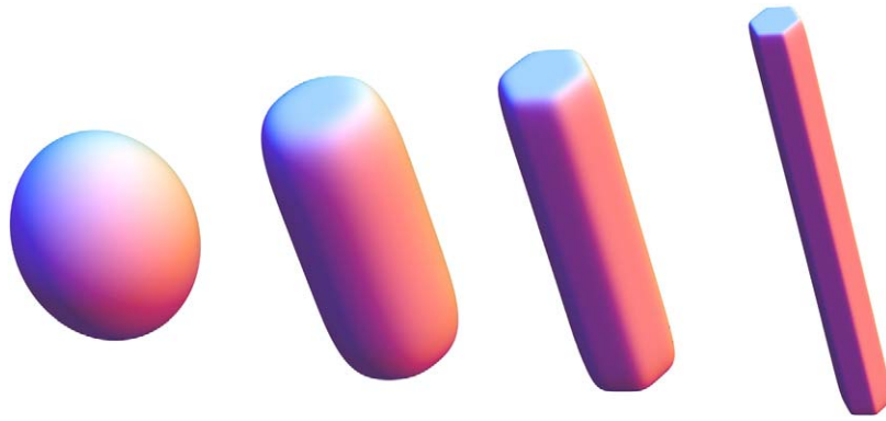
Fig. 2. Contour of the anisotropic norm \ell^p(x)=1 with increasing exponents p=\{2, 5, 10, 20\} and aspect ratios: the angularity of the grain models increases with increasing values for the exponent p . Natural shapes are obtained by high values, e.g., p=10 \dots 20 and L/B=3 \dots 10 . The left contour is an ellipse, i.e., an Euclidean norm for p=L/B=2 .
