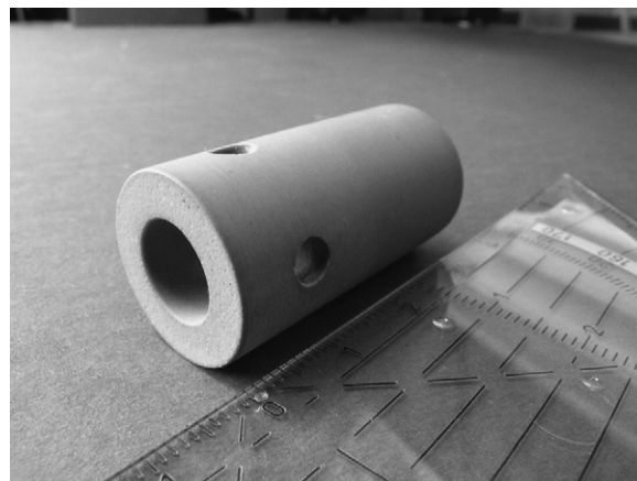
Fig. 6. Cold isostatically pressed, \text{Si}_3\text{N}_4 + 20 wt.% ABSE derived component after crosslinking, green machining (turning, drilling of holes), ceramization and subsequent gas pressure sintering (1800 °C, 1 MPa \text{N}_2 atm).
